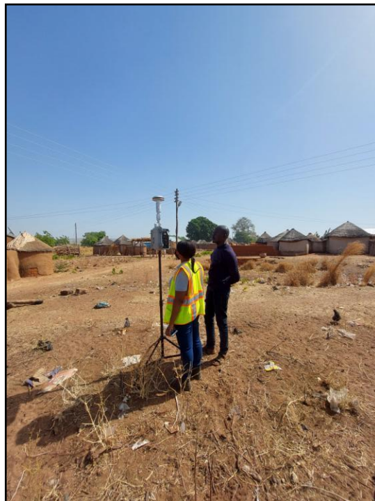
Plate 1: Setting up ARA N-FRM sampler for Ambient Air Quality Monitoring
