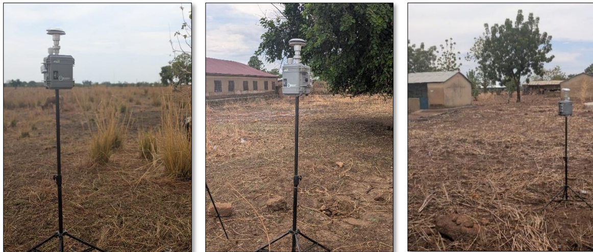
Plate 5-2: ARA N-FRM Setup for PM 2.5 and PM 10 sampling (site -left, school – middle and household – right)
