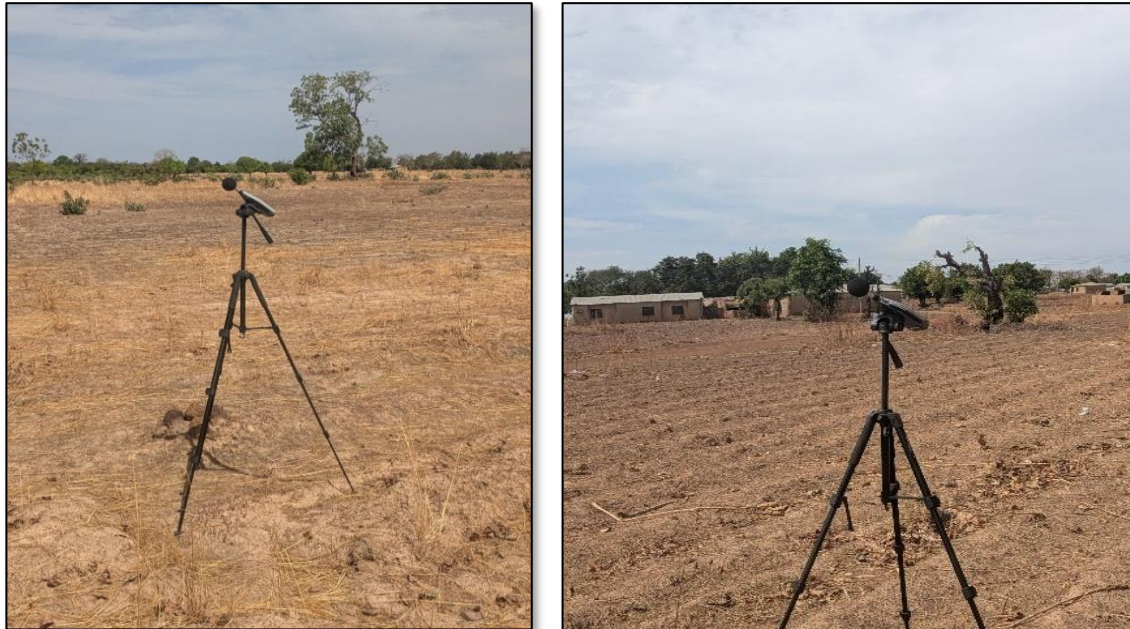
Plate 5-10: Ambient Noise monitoring at the proposed valley and nearest sensitive receptors (SAL Consult, 2025)
