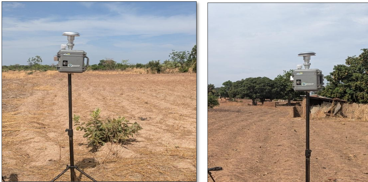
Plate 5-8: ARA N-FRM Setup for PM 2.5 and PM 10 sampling at the proposed Ko rice valley and nearest sensitive receptor (household)
