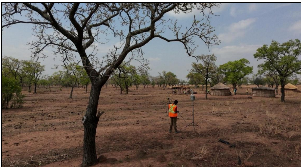
Plate 5-3: ARA N-FRM Setup for PM_{2.5} and PM_{10} sampling at the nearest sensitive receptor (Fulani hamlets)
