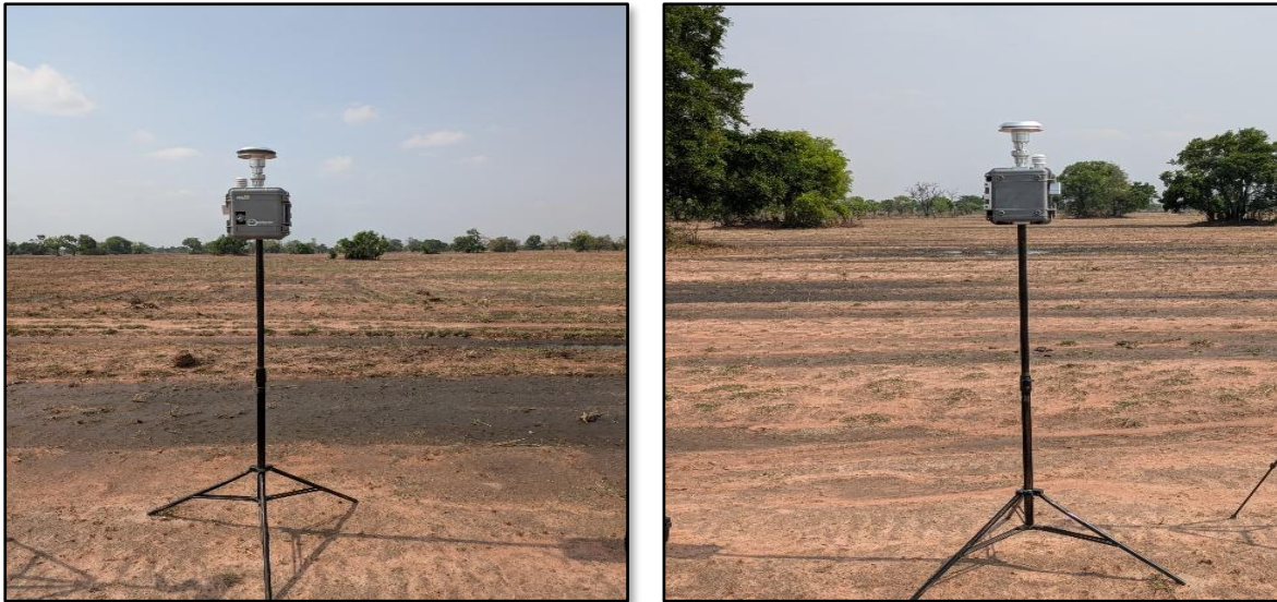
Plate 5-2: ARA N-FRM Setup for PM_{2.5} and PM_{10} sampling at the proposed Nakpanzoo rice valley (SAL Consult, 2025)
