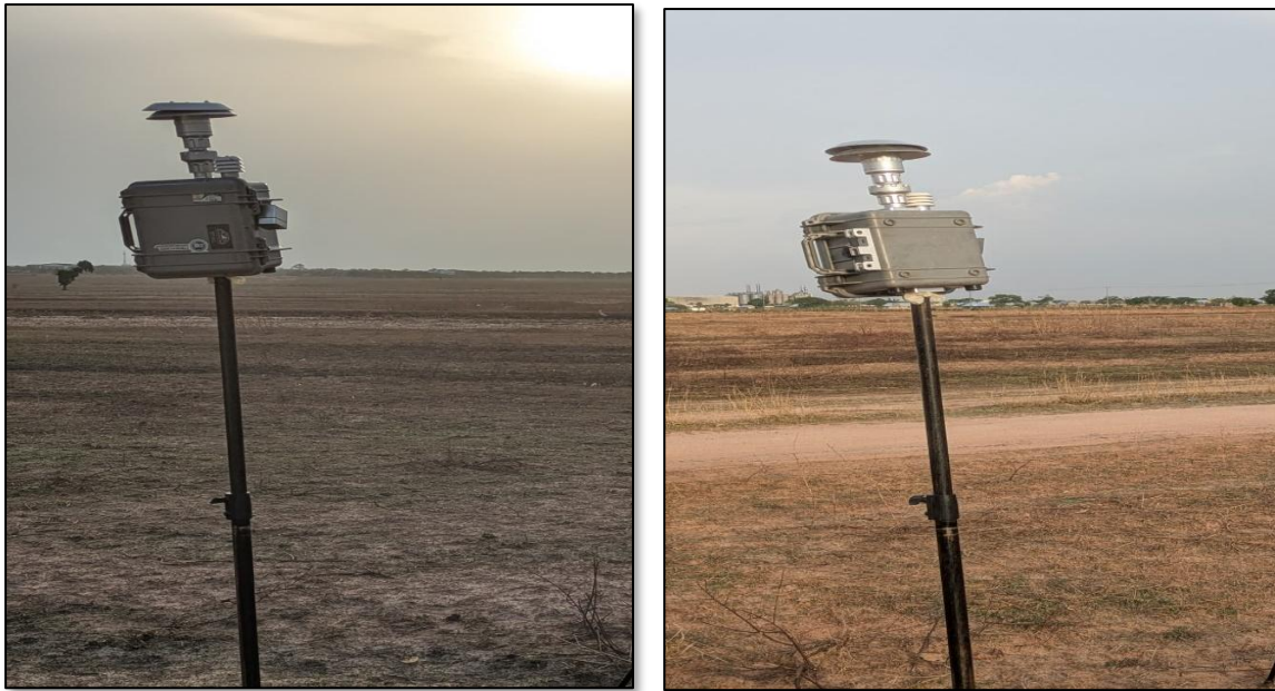
Plate 5-2: ARA N-FRM Setup for PM 2.5 and PM 10 sampling
