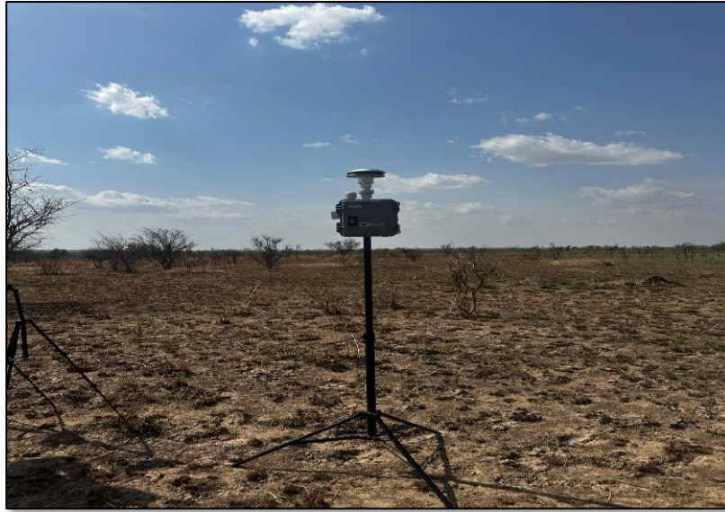
Plate 5-2: ARA N-FRM Setup for PM 2.5 and PM 10 sampling
